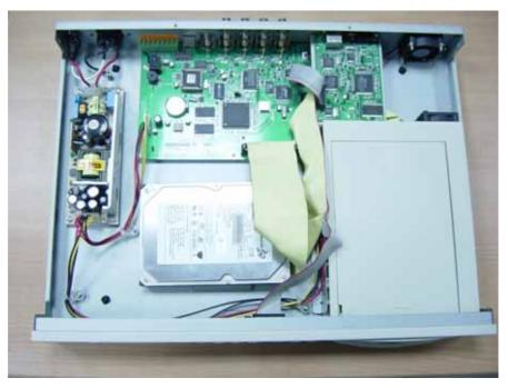
**7.** Restore top cover then hook up with power and monitor a hard drive status message will appear if it's been installed successful.
